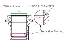
Install retaining ring into retaining ring groove.
