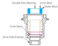
Install double row bearing by pressing on inner and outer race while supporting the inner race of the single row bearing using drive-side endcap.
